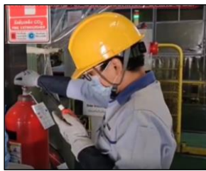
Fig No. 2 Suppress by fire extinguisher (CO2) after cut off electricity of Oiler
